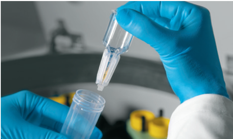
Disposable Ultrafiltration device for sample concentration
